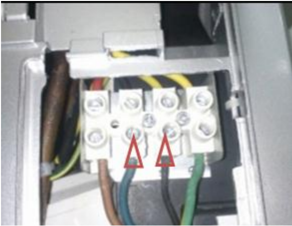
Pic 1: check the voltage of N to S (Vs), is it moving alternately between positive value and negative value?
