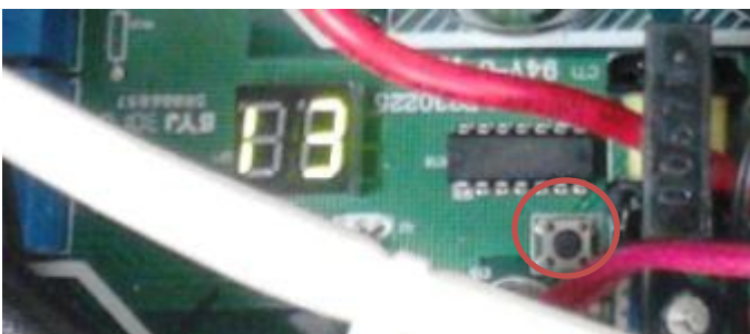
PIC 5: check point button, Press 1 time for check how many indoor units are connected
